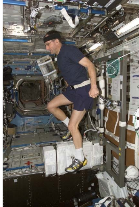
Figure 2d: The Cycle Ergometer with Vibration Isolation and Stabilization System (CEVIS) in use on the International Space Station. (NASA photography)
