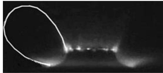
Fig2 : The electric discharge is blown away by the magnetic field gradient
