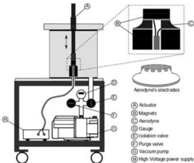
Fig.6 : Experimental device for low pressure MHD experiments.
