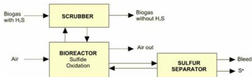
**Figure 4. Biogas desulphurization unit combining an alkaline scrubber with a partial oxidation of HS<sup>-</sup> and alkalinity recovery.**
